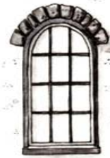
(Fig. 6) Arched Window with Natural Stone Cap
