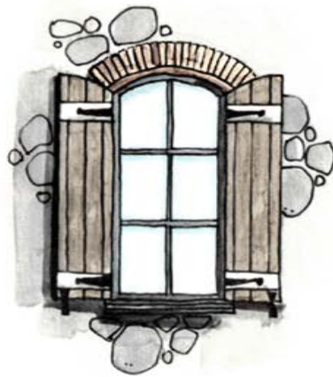
(Fig. 5) Arched Window with Wooden Shutters and Brick Cap
