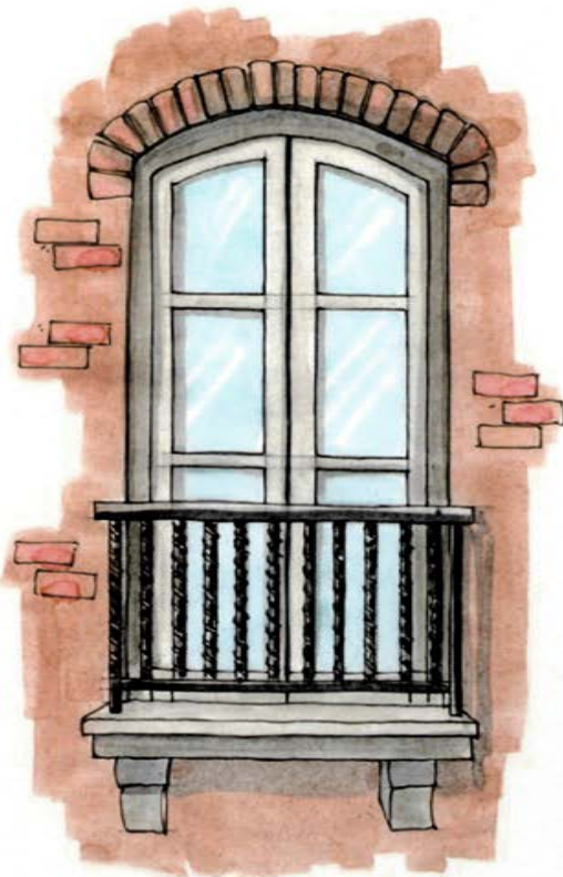
(Fig. 2) Balcony with Turned Wrought-Iron Rail
